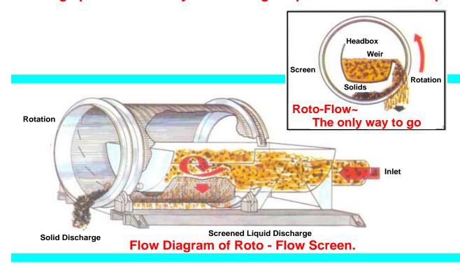
The importance of the ROTO-FLOW technology is in introducing the liquid at 90 relative to the lie of the wedge wire. This is used for the initial separation of solids from liquid & in all cases the effluent liquid is introduced tangentially on to the contra- rotating face. The screen will discharge over only one weir as discharge over more than one can cause excessive moisture at the bottom of the screen drum with the attendant problems of loss of efficiency & screen blinding.
